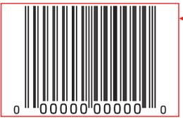
Bounding box to show minimum clear area for 80% UPC. Minimum clear area is 9 times the width of the narrowest bar or space in the barcode.
