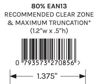
\*Barcodes may be truncated to a reduced height. We do not recommend less than .5" high. The width should remain as shown above in "suggested clear zone" and never less than the "minimum clear zone"
