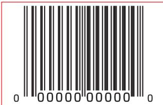
Bounding box to show minimum clear area for 100% UPC. Minimum clear area is 9 times the width of the narrowest bar or space in the barcode.
